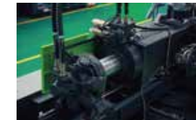
Single-cylinder injection structure
