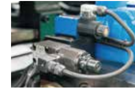
Proportional valve-controlled back pressure
