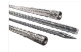
High mixing anti-stick screw design
